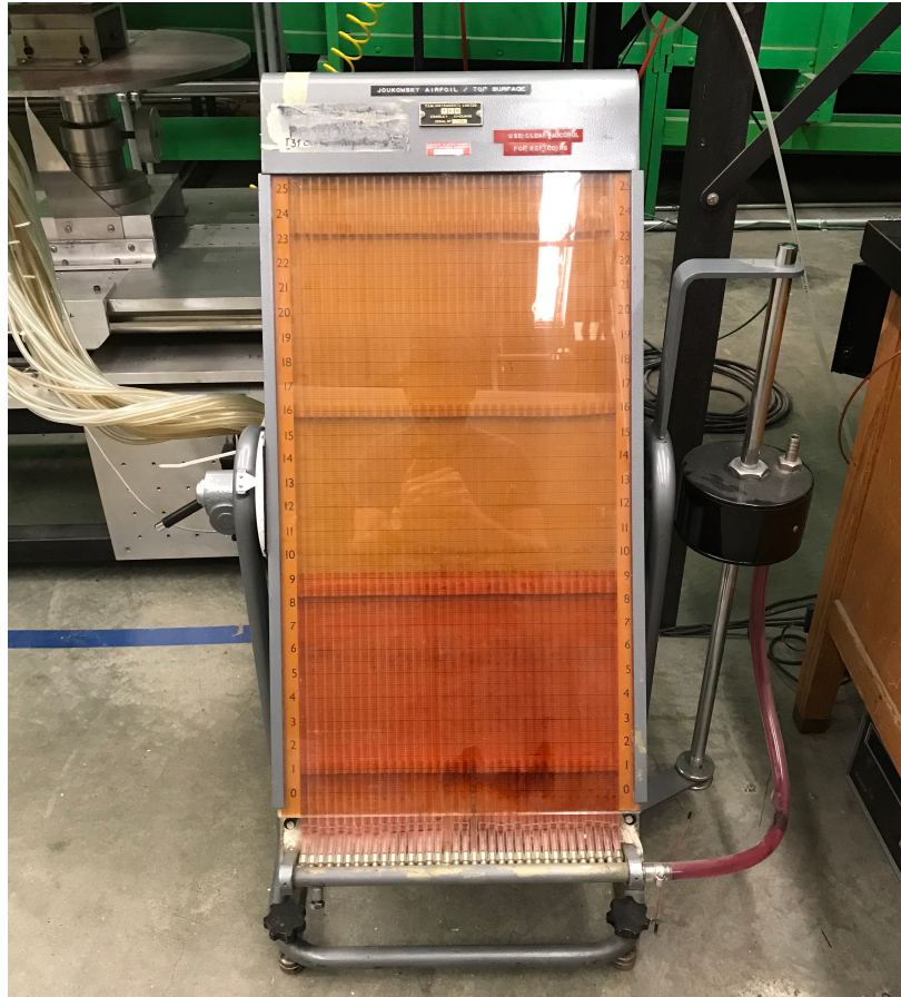
Figure 6: Multi-tube manometer filled with Ethyl Alcohol.
