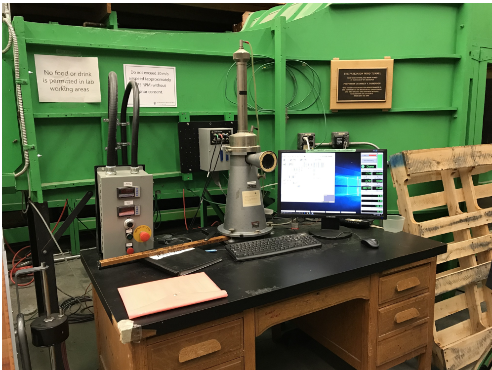
Figure 2: Data acquisition, fan controller, and Betz manometer.
