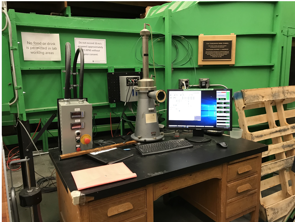
Figure 3: Data acquisition, fan controller, and Betz manometer.
