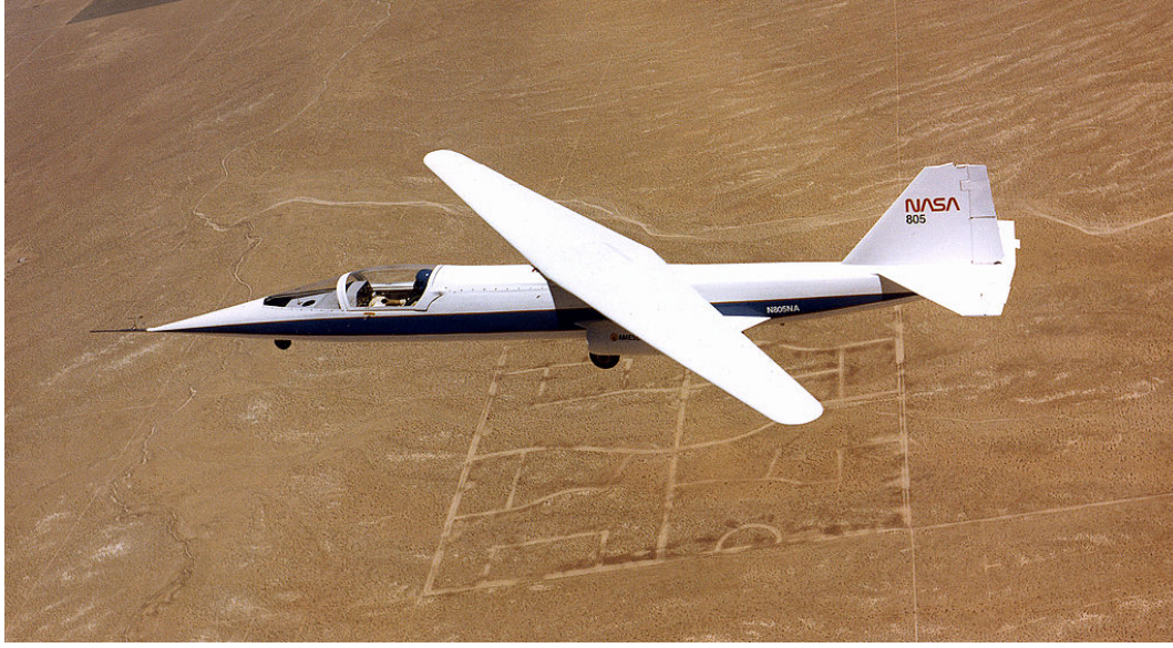
Figure 4: The AD-1 oblique wing research aircraft (courtesy of NASA Photo ECN 13305-4).
