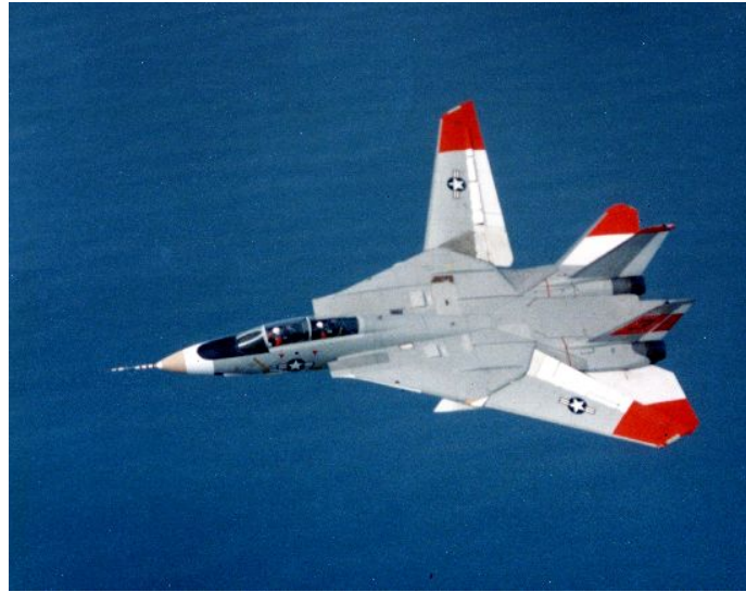
Figure 1: A Grumman F-14 Tomcat during a test of an unusual asymmetric wing configuration (courtesy of San Diego Air & Space Museum Archives).
