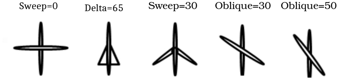
Figure 6: Five different configurations of wings flying at Mach = 0.9 [5].
