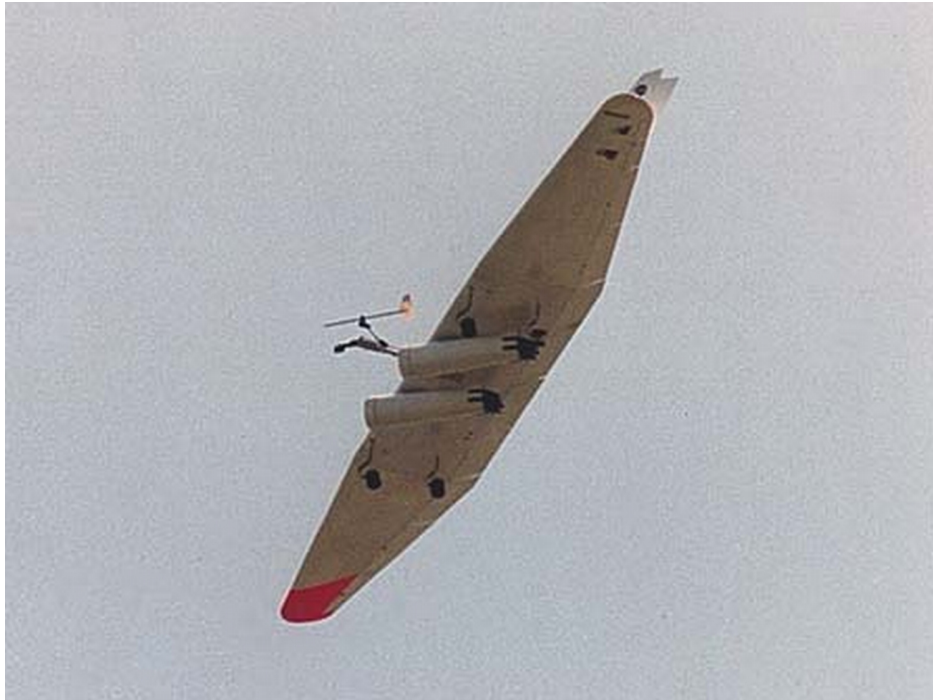
Figure 10: An oblique all wing aircraft model [8].
